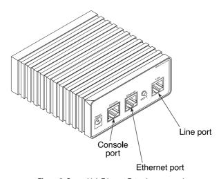
Figure 2. CopperLink Ethernet Extender rear panel
